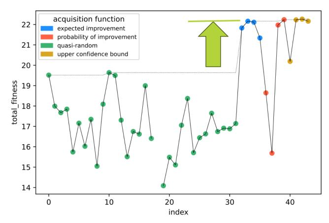
Above: optimizing the flux density of the KB mirror system of the simulated TES beamline (4 dims). After 32 random initialization points, we rapidly find the global optimum. This takes 2-3 minutes at the real TES beamline. The fitness is log-scaled, so ~20 times more flux density than at the start.  ${}^9$ o
