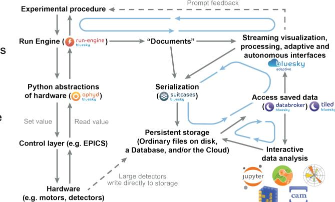
Data acquisition system for high-level control and planning
